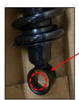
Incorrect part Bushing and sleeve missing
