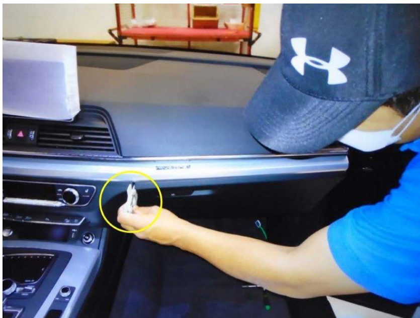
Figure 3. Checking the gap between the glove box door and the center console.
