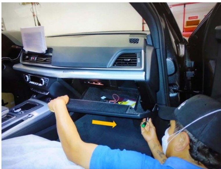
Figure 2. Adjusting the glove box to increase clearances.
