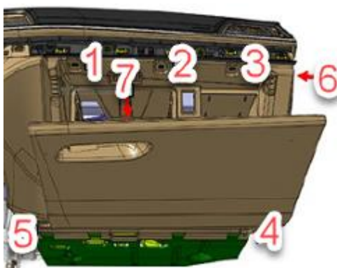
Figure 1. Glove box bolt tightening sequence
