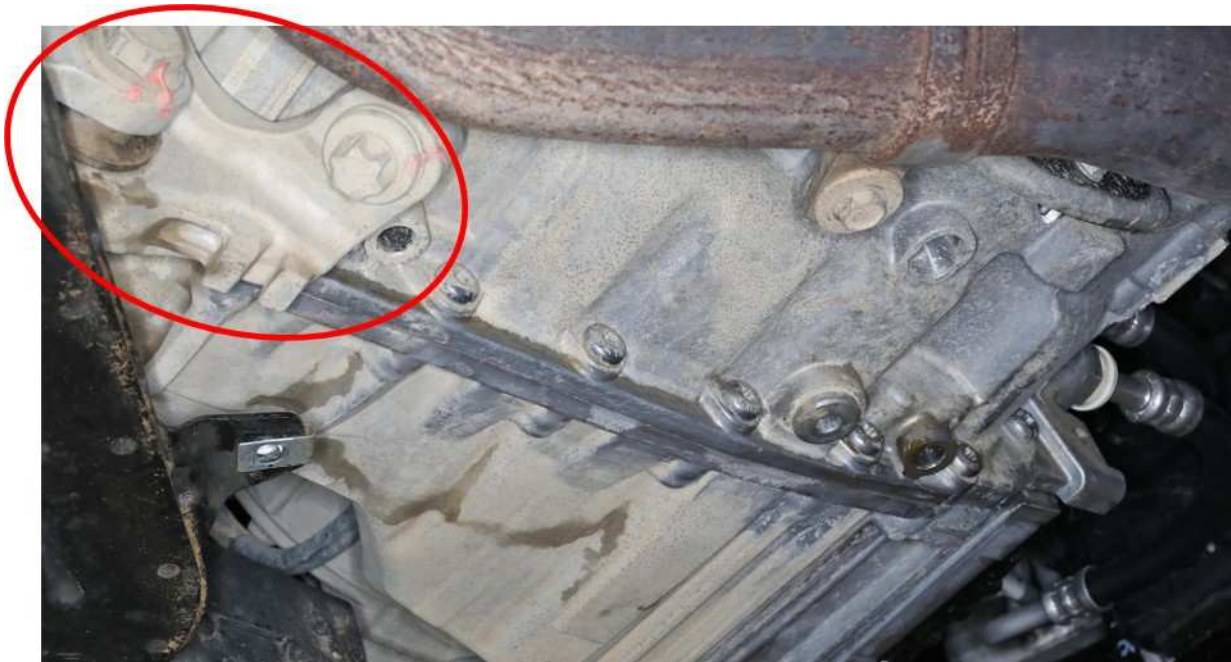
Fig. 3 Support Bracket to be Removed
