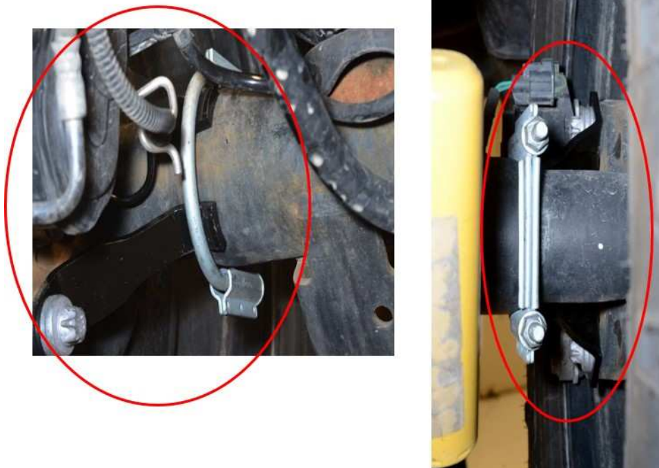
Fig. 4 Brake Brackets and U-Clamp Installed
