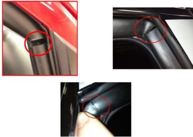
Fig. 1 Examples Of Weatherstripping Splits And Tears
