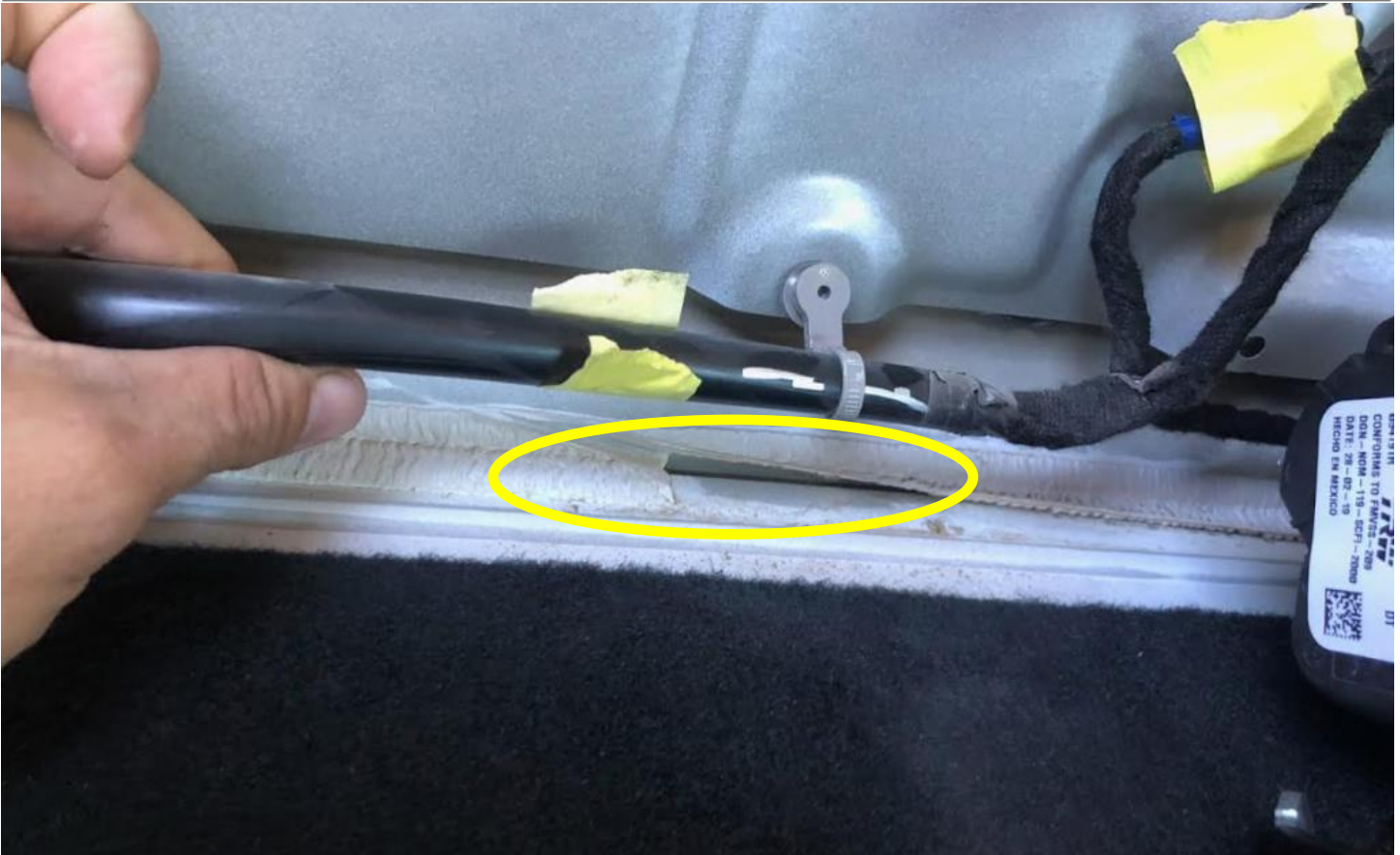
Fig 2. Rear cab floor to bulkhead sealer. Sealer gap shown circled.
