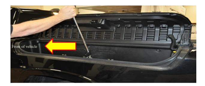
If the gap is higher at the REAR, open the lid and carefully use a MOPAR essential tool 2069900230 to bend the striker forward (toward front of the vehicle).
