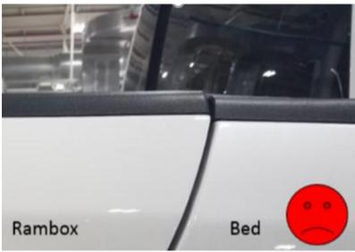
If the lid is over flush to the bed trim at the top, open the lid and use the striker tool to bend the striker DOWN. After adjusting, evaluate closing effort and fine tune as needed.
