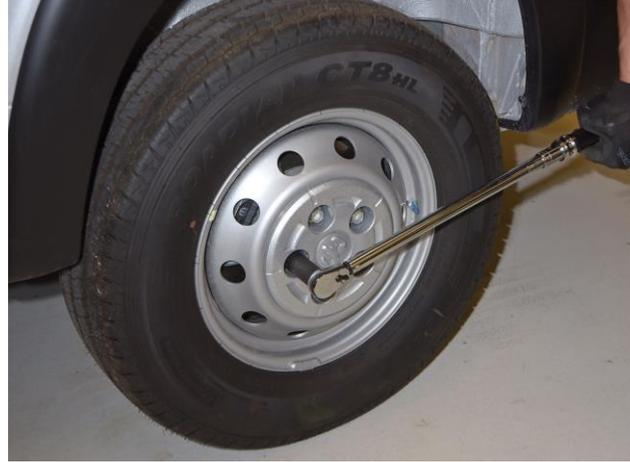
**Figure 7 – Torque Wheel Bolts**
