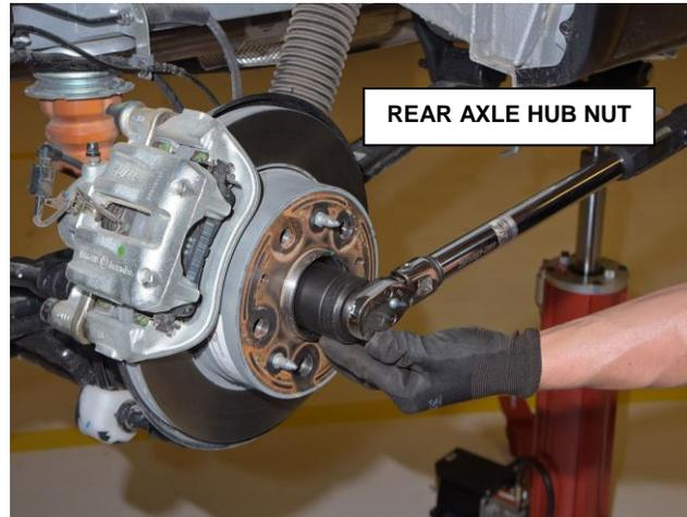
**Figure 3 – Rear Axle Hub Nut**
