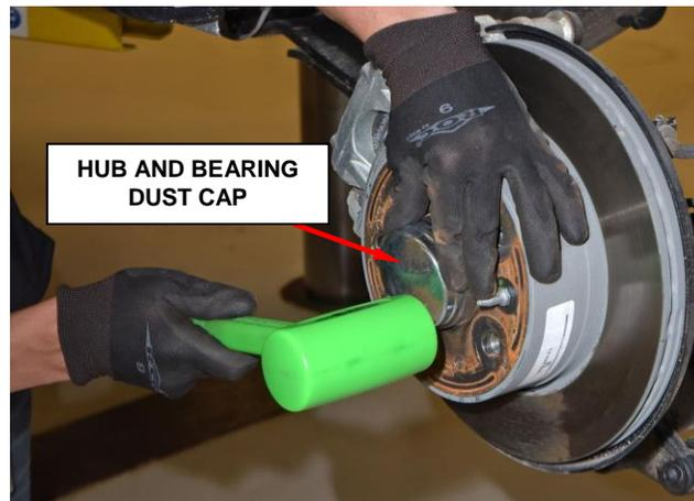
**Figure 6 – Hub and Bearing Dust Cap**
