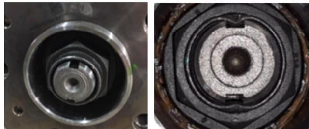
Figure 2 – Un-Crimped and Crimped Nut
