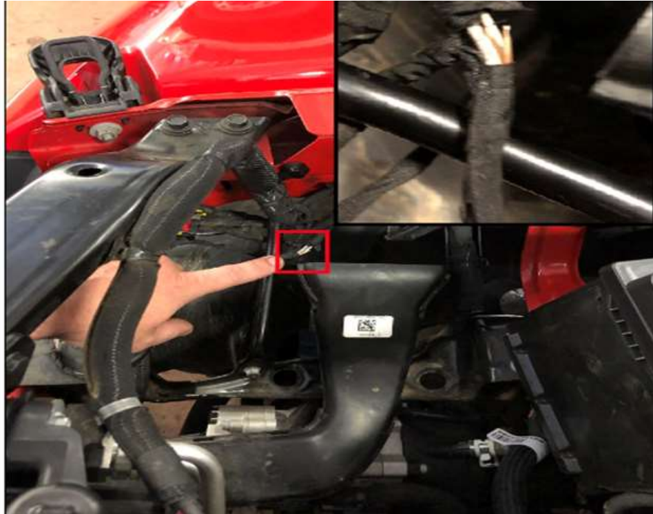
Fig 2, suspect harness stretch area.
