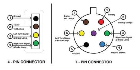
These graphics represent typical tow vehicle wiring configurations. Wire colors can vary depending upon the manufacturer. It is recommended to always use a circuit tester to verify connections.
