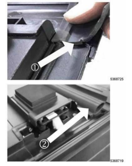
**Important:** Verify the front tonneau cover seal is the revised "fin" style seal (1). If the "bulb" style seal is installed (2), replace the seal. Refer to steps 1-5 of the Adjustment Instructions for Vehicles That Have NOT Had Recall N192217500 performed below.
