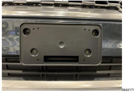
2. Install the new front license plate bracket using the diagram above.
