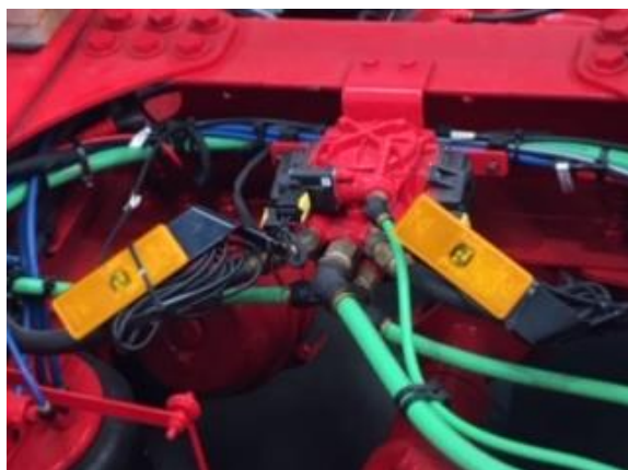
Left: Side marker lamps, brackets and wiring bundled to chassis
