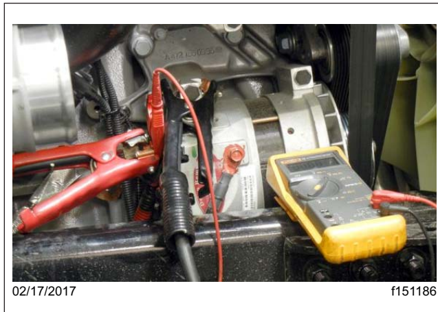
Fig. 5, Alternator Positive Cable Check
