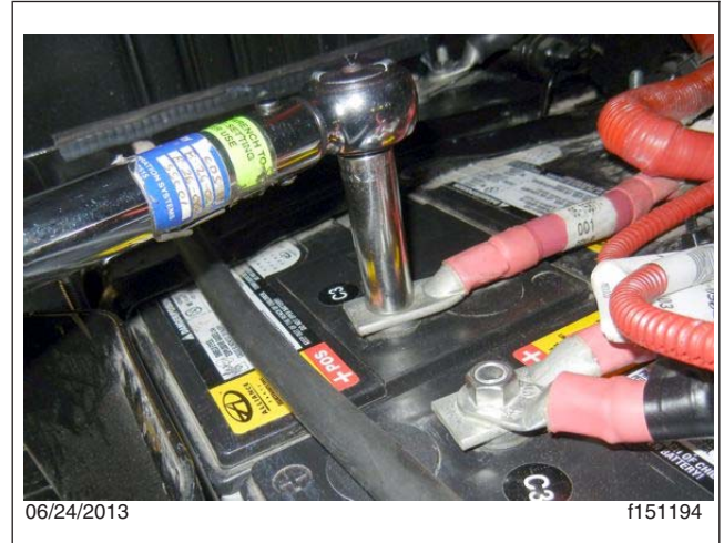
Fig. 11, Check the battery connections for looseness and corrosion. Check the torque on the connections.
