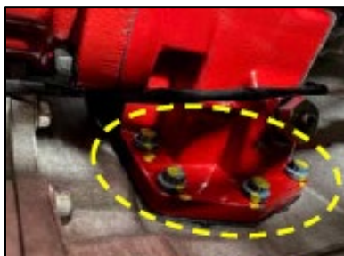
Figure 1. Witness Marks on PTO Mounting Screws and Flange
