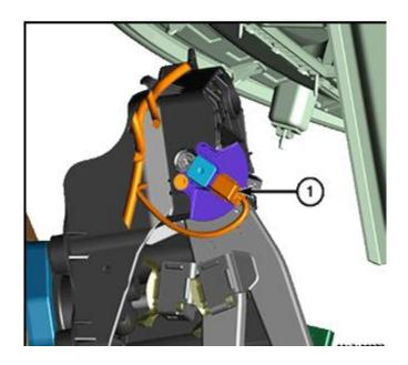
Inspect brake pedal sensor (1), secure sensor to bracket and perform the brake sensor calibration procedure using the scan tool procedure under PCM to complete.
