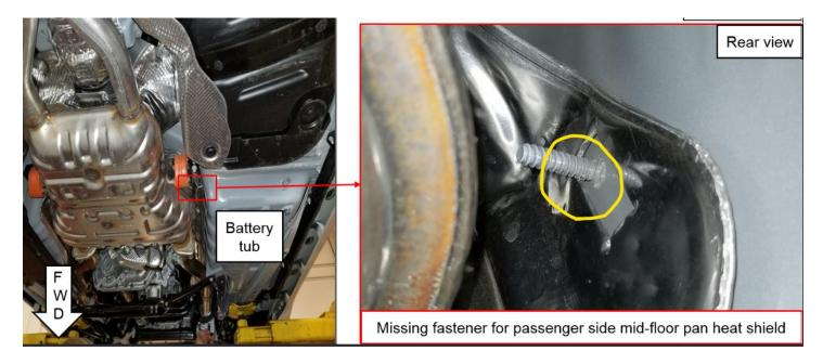
Inspect under body heat shields for contacting power train/driveline items. Also look for any missing retainers or fasteners. See the above images.
