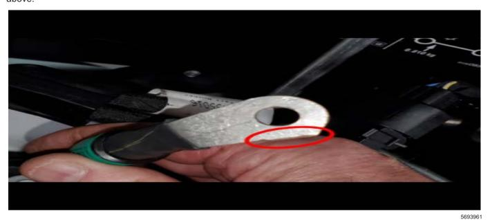
Important: DO NOT cut the all the anti rotation tab flush, as shown in the graphic above. Cutting the tab flush may cause the cables to rotate and contact the
