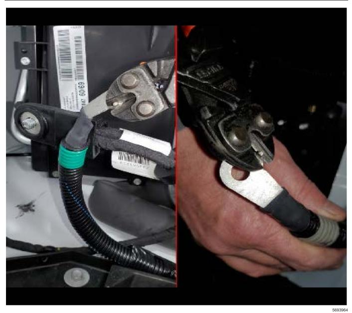
5. Utilizing cutters, cut the tabs from the cables.
