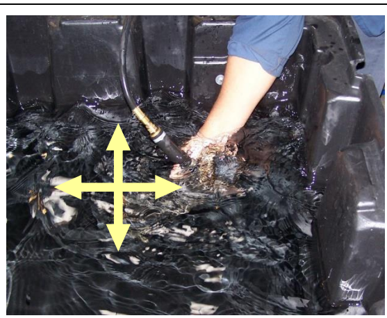
Shake Cooler to release trapped air
