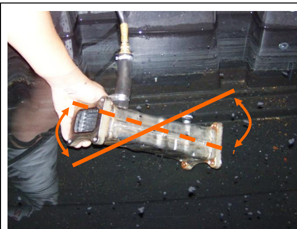
Rotate Cooler to release trapped air
