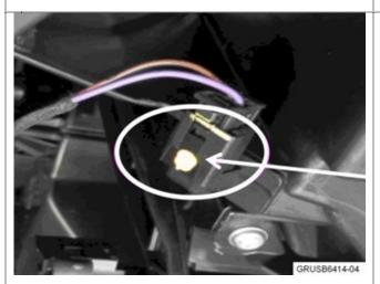
7. Check for a marking on the electrical connector.
