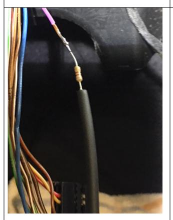
Make sure to place the heat shrink tubing over the wire before you install the resistor.
