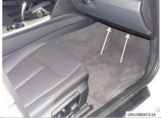
1. Remove the passenger's side footwell cover trim (the bottom instrument panel trim).
