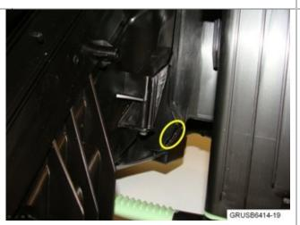
5. The close-up picture shows the exact location (circle) of the sensor opening. The following steps will be performed from the lower passenger's footwell area at the bottom of the IHKA housing.
