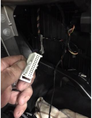
Remove the outer plastic housing from the internal wire holder to identify the wire you will be modifying.
