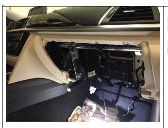
Removal of the glove box and knee airbag makes access to the wiring harness easier for installation of the resistor.
