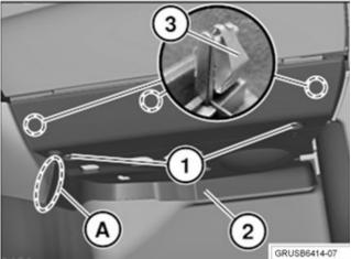
2. Remove both screws at connection (1).
