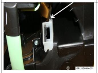
8. Insert the new adapter firmly into the sensor opening, as shown.
