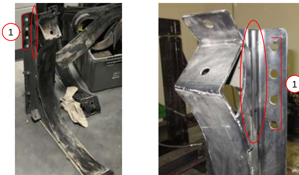
Figure 1. Clean corner bends (circled) adjacent to mounting holes (1) on front of brackets. NOTE: Brackets shown uninstalled for clarity.
