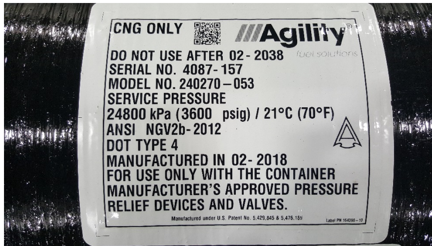
Figure 7. Cylinder manufacturer label must be in place and legible. Verify label is not expired and cylinder is correct for CNG use.
