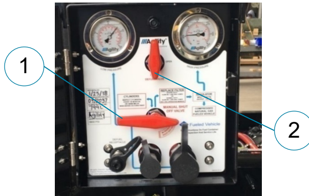
Figure 48a. Box style FMM with red 1/4-turn manual shutoff valve (1) and defuel valve (2) on FMM front panel.
