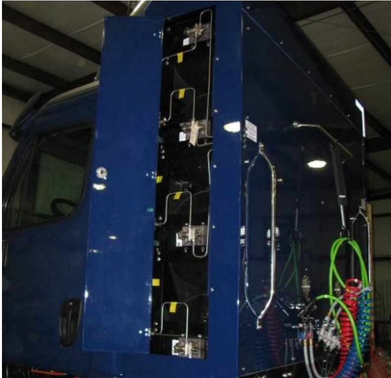
Figure 22. Typical behind the cab (BTC) fuel system cabinet.
