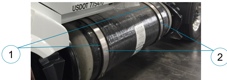
Figure 43. Cylinder brackets, straps and rubber isolators must be in place and secure. Rubber isolators (1) must be centered beneath the straps (2) and brackets (not visible) and must not be displaced or distorted on the mounts.
