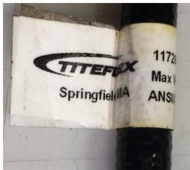
Figure 31. Left: Titeflex plastic coated paper tag may or may not be present. Right: Titeflex hose outer jacket is imprinted with “TITEFLEX” branding, date of manufacture (circled), and maximum pressure and temperature range ratings. NOTE: Hose sample shown for illustration purposes; markings will vary with application.
