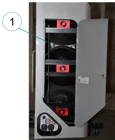
Figure 24. Back of cab system showing area PRD trigger line (1) behind the side door. Similar trigger lines are routed on the opposite side.
