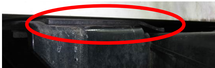
Figure 38. Rubber isolator (circled) between the BTC cabinet and vehicle chassis on a four year old system with 316,000-plus miles. A quick look indicates the rubber pad is in good condition.
