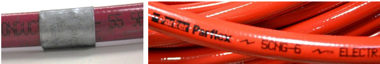
Figure 33. Left: Parflex 5CNG hose metal ID tag includes a plant code, manufacturing location, and manufacturing date code (not visible).
