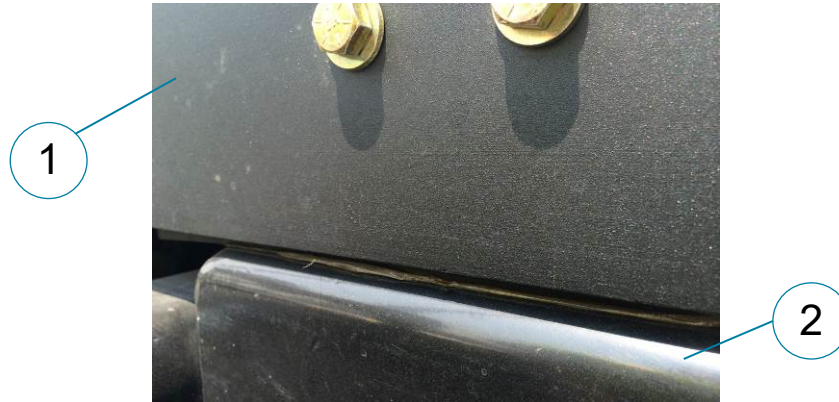
Figure 39. There should be no metal to metal contact between the mounting bracket or vehicle chassis (1) and fuel system cabinet. (2)
