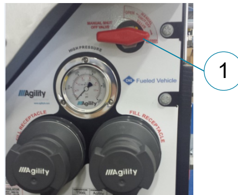
Figure 49b. Back of cab FMM panel with red 1/4 turn manual shutoff valve (1) on FMM front panel; NOTE: 1/4-turn defuel valve (not visible) is inside fuel system cabinet.
