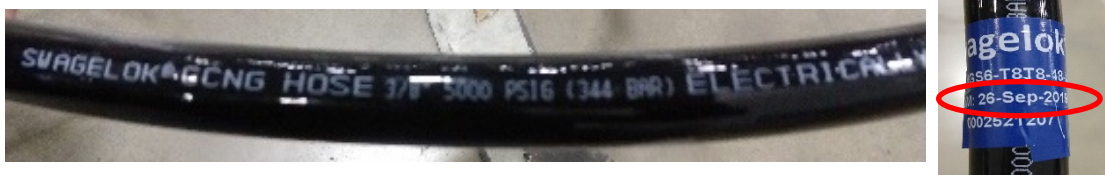
Figure 35. Left: Swagelok NG Series hose outer jacket marked “SWAGELOK®” with size and pressure rating and “ELECTRICALLY CONDUCTIVE”. Right: Swagelok hose decal includes date of manufacture (DOM) (circled).
