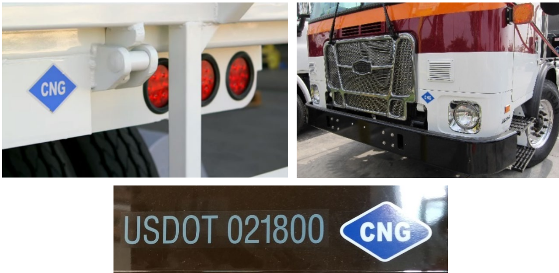
Figure 9. Left: Compressed natural gas powered vehicles are identified by a blue and white CNG diamond decal on the right rear and both sides of the vehicle power unit.
