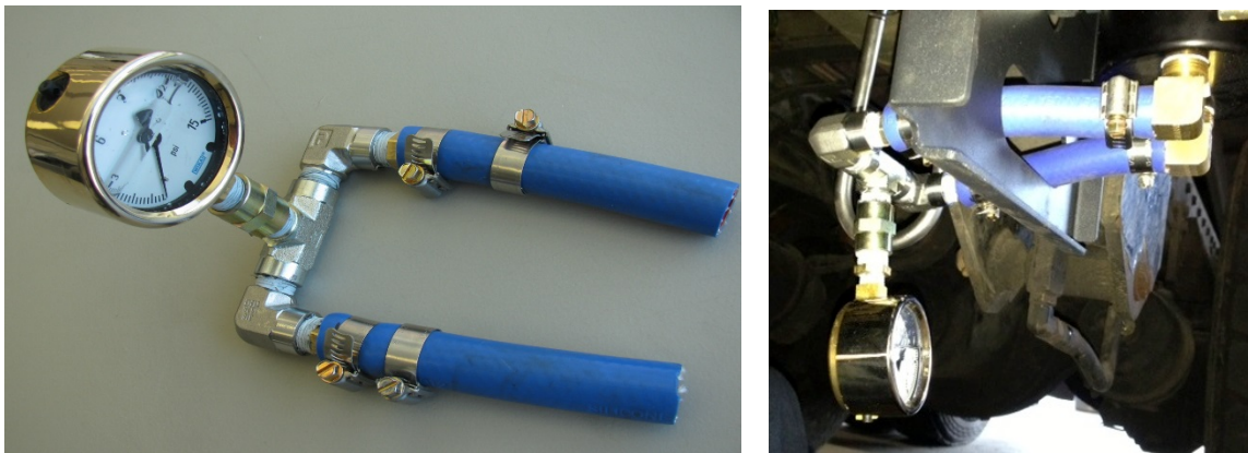
Figure 60. Left: Shop-built pressure regulator test jig. Right: Test jig installed on pressure regulator coolant inlet and outlet ports.
