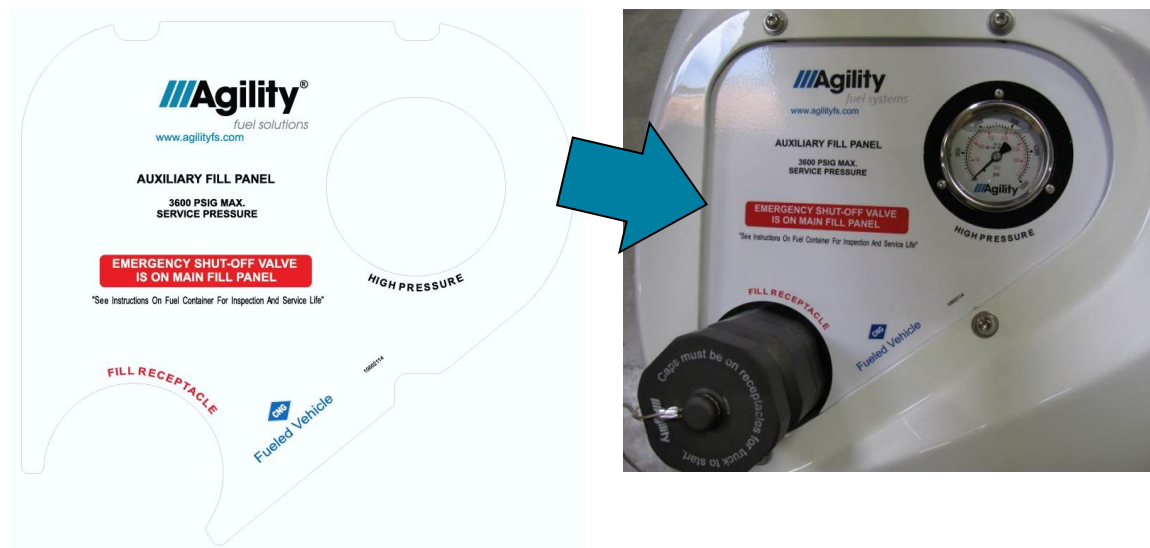
Figure 13. Auxiliary fill panel decal. Blue arrow indicates warning message directing operators and first responders to 1/4 manual shutoff valve located on main fill panel.
