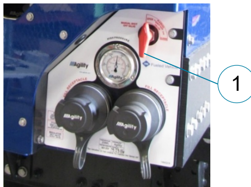
Figure 46b. Box style FMM with red 1/4-turn manual shutoff valve (1). The 3-way defuel valve (not visible) is accessed from the bottom of the FMM chassis box. Refer also to Figure 6.
