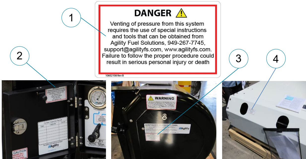
Figure 14. Place “Danger high pressure” decal (1) in multiple locations: inside FMM (2), on cylinder enclosures (3), adjacent to pressurized lines (4) and near cylinder and bleed valves (not visible).
