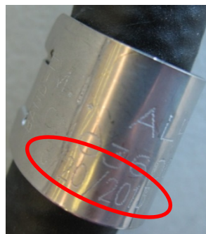
Figure 29. Motion Industries CNG hose metal ID tag includes date of manufacture (circled).
