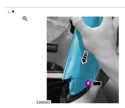
Apply downward pressure onto the windshield molding and fully tighten the retaining bolt.
