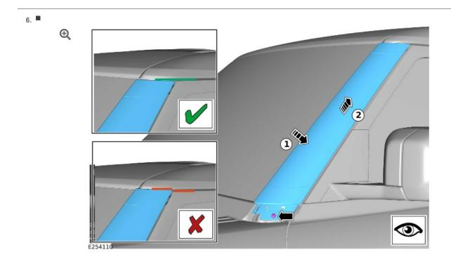
Install the windshield molding in the directions shown.
