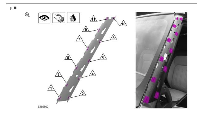
Locate the 11 windshield molding retaining ribs as shown highlighted.
