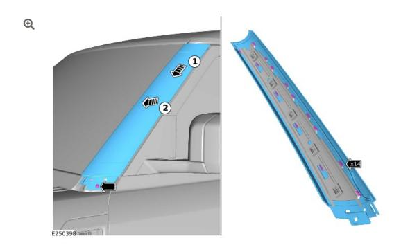
Remove the retaining bolt and then remove the windshield molding.
