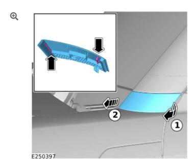
Release the 2 clips to remove the windshield molding bolt cover.
