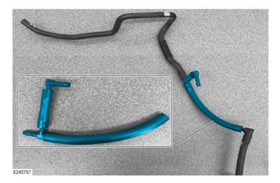
Install the section of active engine mount vacuum hose, as shown in the illustration.
