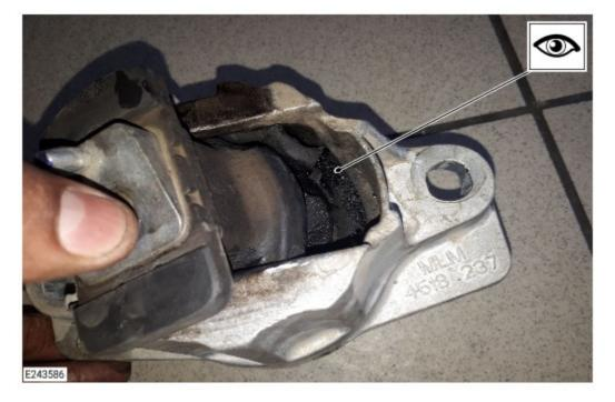
Example photograph of an excessively worn and/or leaking active engine mount.
