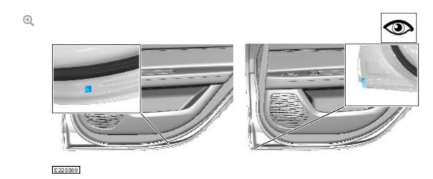
Inspect the rear door(s) inner and outer drainage aperture(s) for any excess sealant obstructing the drainage aperture(s).
