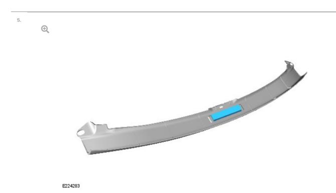
Install the double-sided self-adhesive foam to the luggage compartment header panel trim.
