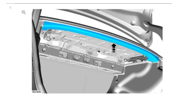
Apply firm pressure to the center of the luggage compartment header panel trim to make sure the self-adhesive foam has bonded.
