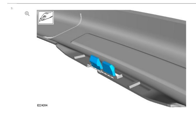
Use a suitable tool to cut the retaining clips from the luggage compartment header panel trim.
