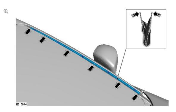
At the 6 positions shown, close the internal dimension of the windshield finisher retaining channel on the A-pillar.
