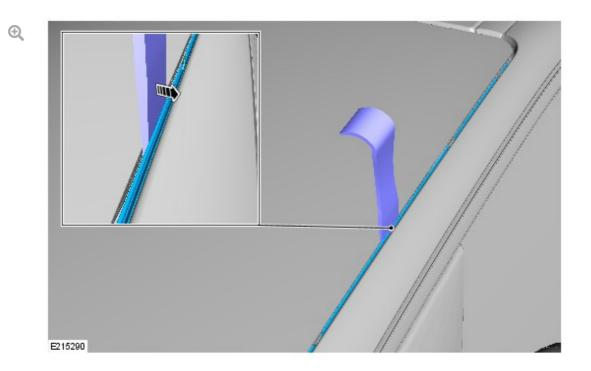
Insert a suitable, 30-40mm-wide plastic tool and pull towards the A-pillar.
