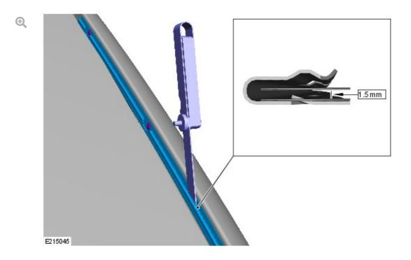
Close the windshield finisher channel to an internal dimension of 1.5 mm.
