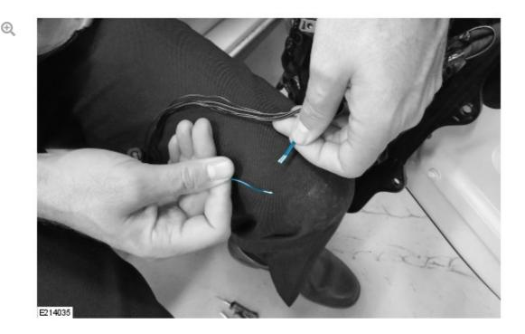
Cut the repair wire to a suitable length and prepare the front right door electrical wiring harness for a splice connector.
