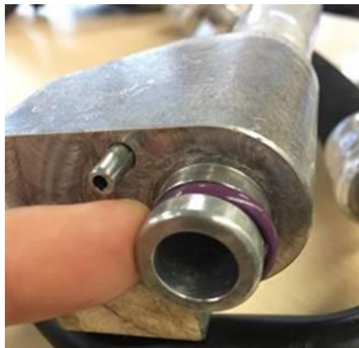
Figure 1. Damaged refrigerant line O-ring seal.
