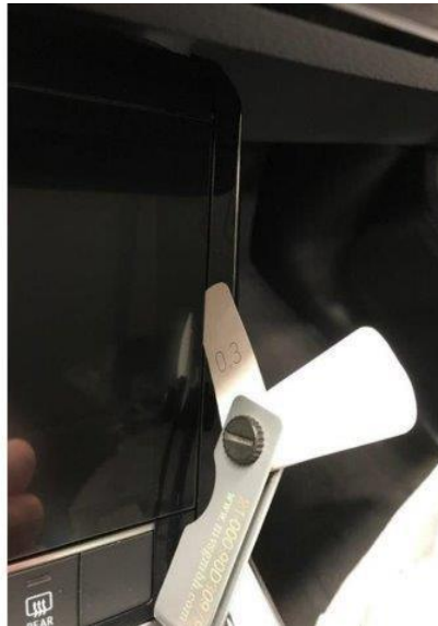
Figure 4. 0.3 mm gap after the repair.
