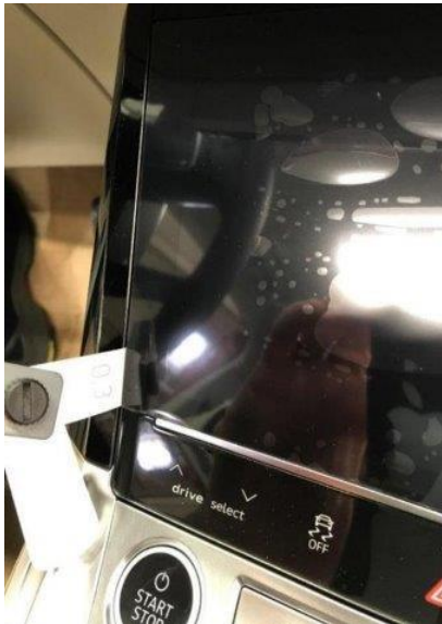
Figure 3. 0.3 mm gap after the repair.
