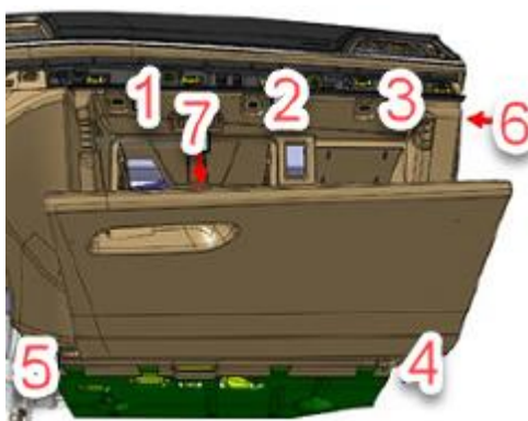
Figure 1. Glove box bolt tightening sequence
