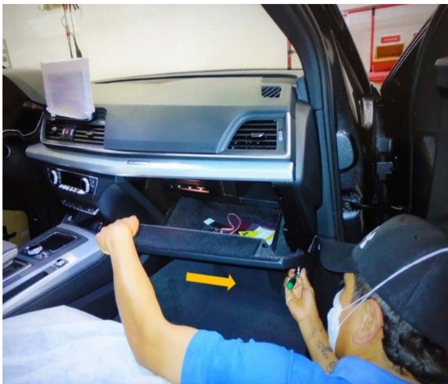
Figure 2. Adjusting the glove box to increase clearances.
