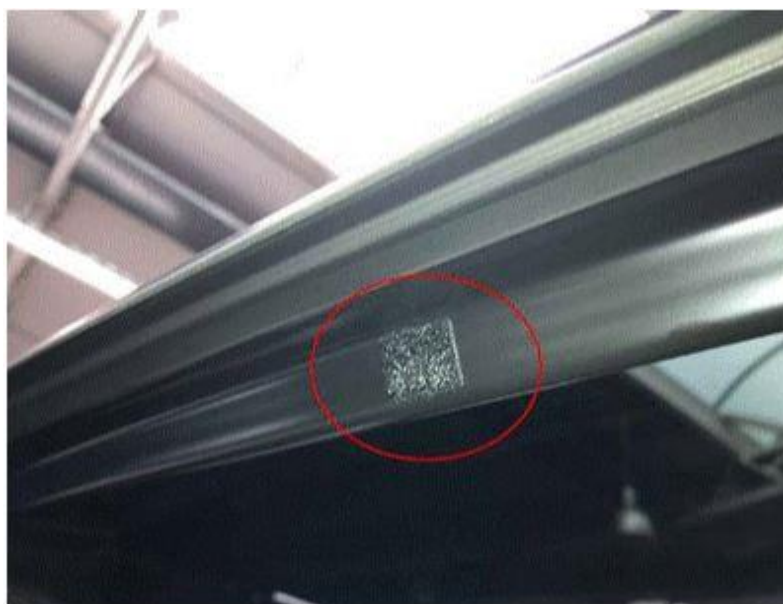
Figure 17. Adhesive felt strip material affixed to the center area of sunroof glass panel structure.
