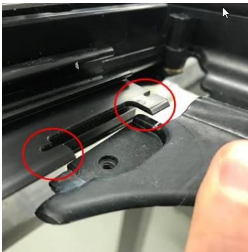
Figure 7. Areas to clean using cleaning solution D 009 401 04.
