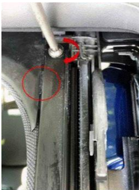
Figure 14. Tightening of the screw with the felt strip material isolating the guide rail and the frame.
