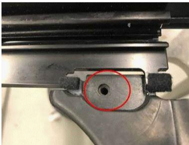
Figure 10. Apply thread locker in this area.
