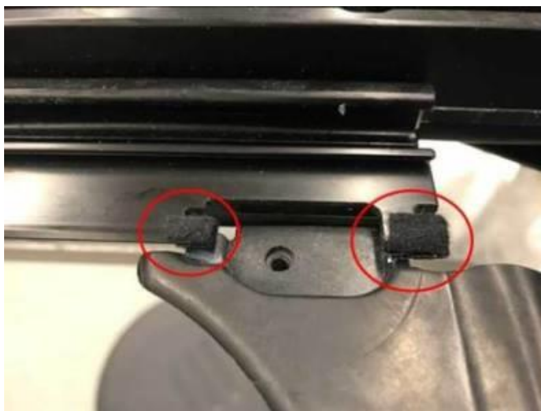
Figure 9. Apply felt tape on points shown. The tops and bottoms of the tabs must be isolated.
