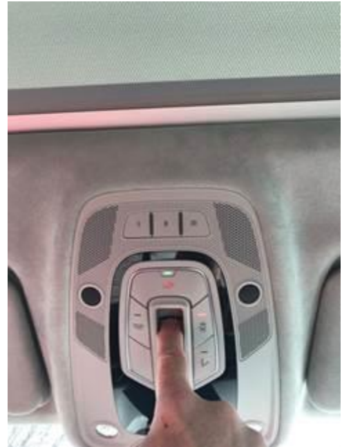
Figure 2. Set the sunroof shade basic settings by pushing the sunroof shade switch fully forward.
