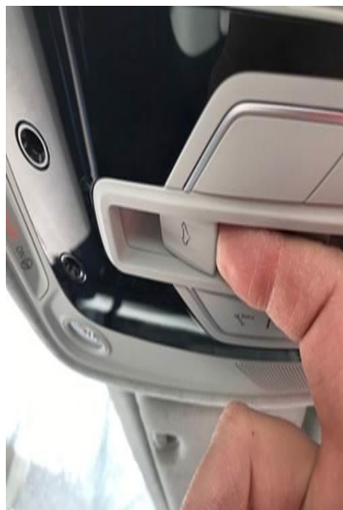
Figure 1. Set the sunroof panel basic settings by pulling the sunroof switch fully downward.
