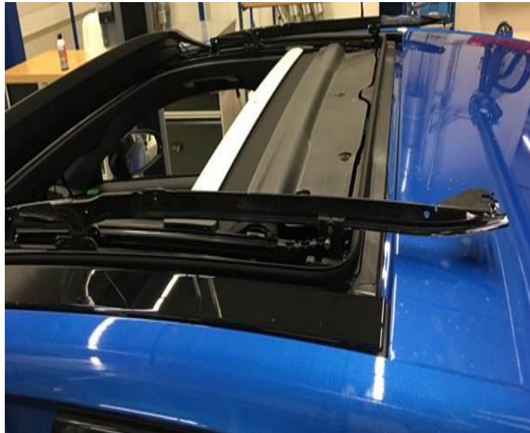
Figure 1. Sliding rails exposed showing the area of contamination.
