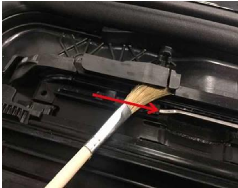
Figure 5. How to apply the grease.
