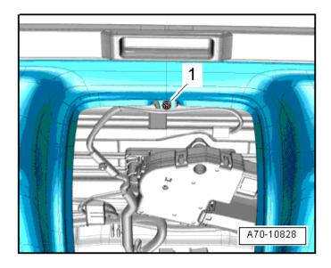
Remove the bolt <1> in the front interior/reading light roof opening.
