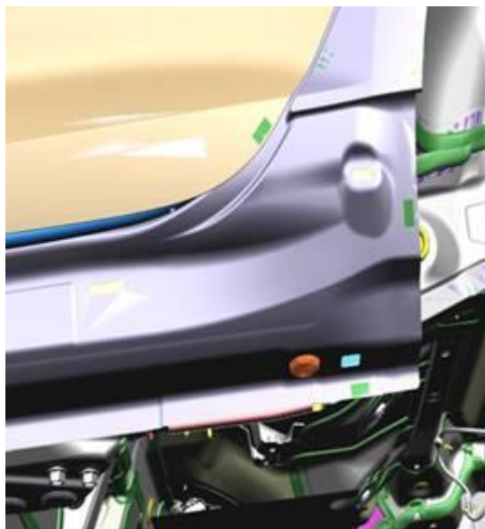
Figure 11. Drain plug on rear of the side member.
