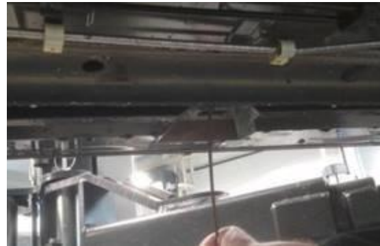
Figure 9. Making the hole in the sound absorber.
