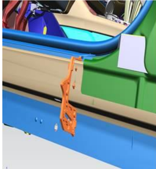
Figure 6. Side member cavity sound absorber.
