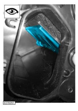
The illustration shows a distribution door in the 'closed/up' position. If a distribution door is in the 'open/down' position, carefully manually close the distribution door.
