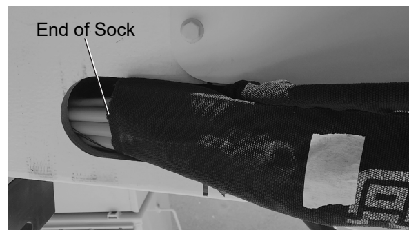
Figure 3 — Pulling Sock Out of Boom
