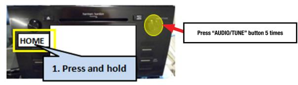
• Switch the unit into "Diagnosis Mode" by pressing and holding the HOME button while pressing the "AUDIO/TUNE" button 5 (five) times.
