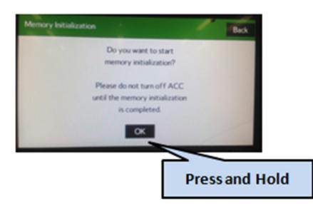
• Press and **HOLD** the "OK" button until the screen shown below is displayed (5 to 10 seconds).
