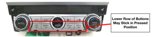
The shape of the control panel body behind the buttons was changed to prevent occurrence of this condition.
