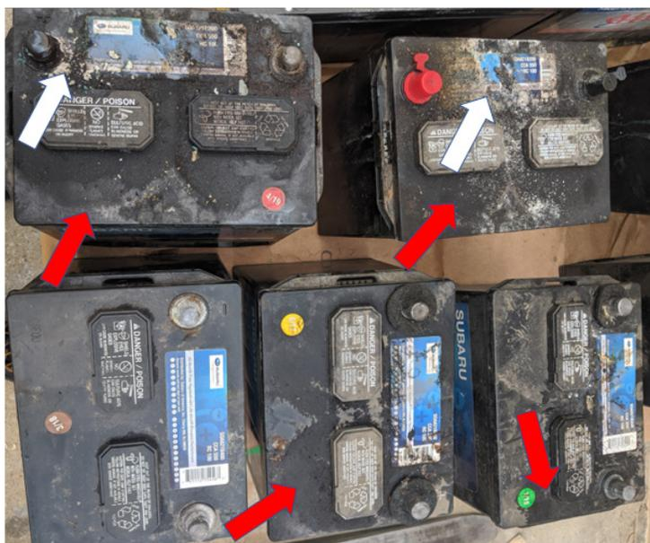
In this collection of returned batteries, the RED arrows point to moisture accumulations which has escaped from either the post seal(s) and / or the covers (fill caps) as a result of normal outgassing, a normal by-product of charging. The two WHITE arrows point to corrosion. Both are normal conditions and not to be considered defects.
