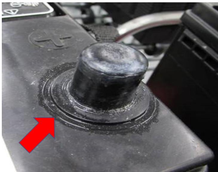
The RED arrow points to moisture seepage seen around the post seal. This photo depicts seepage which should be considered normal and would not be considered a warrantable defect requiring battery replacement.
