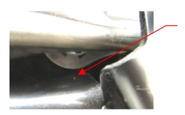
When the Lifter is at the bottom (lowest) position, there is only a very small gap between the Lifter and the Bracket. In some cases, there may be a small "witness mark" created by the contact usable as a guide for where grease must be applied.
