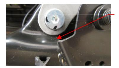
When the Lifter is at the top position, there is space between the Lifter and the Bracket.
