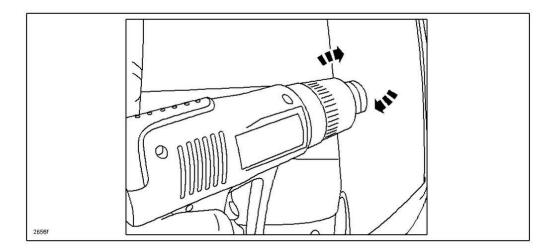
Once the upholstery material reaches a warm temperature, use the pre-soaked cloth to apply firm hand pressure in a outward motion.
