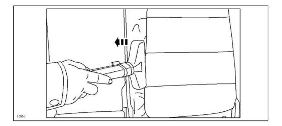
If necessary, use your hand to work out the seat wrinkles by applying firm pressure in a outward motion. This step can be repeated as long as the upholstery material is warm. If the upholstery material feels cool, re-apply steam.
