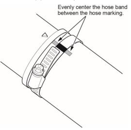
9. Tighten the hose bands to the specified condition below.
