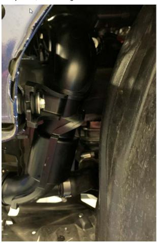
8. Slide the intercooler outlet hose onto the intercooler outlet pipe assembly. Then, install the hose band into position by lining up the paint mark, and the mark on the intercooler outlet pipe assembly.
