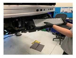
7. Transfer the mounting hardware. Then, install the intercooler outlet pipe assembly to the vehicle, and torque the two bolts to **9.3 N.m (6.9 lb-ft)**.
