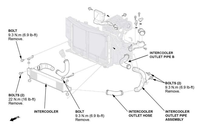
4. Remove the intercooler outlet hose.
