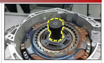
14. Secure the **SST 09430 2A240** (J) onto the clutch housing as shown and then turn the bolt head clockwise until the dual clutch assembly is secured.
