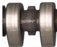
Excessive wear On wetted parts
