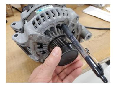
If after inserting the pen or tool, the pulley can spin in both directions, then pulley is bad and the alternator needs to be replaced. If the pulley spins only to left (counterclockwise) with a tool/pen, the alternator pulley is not the issue.
