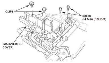
19. Remove disconnect the connectors, then remove the IMA inverter cover.
