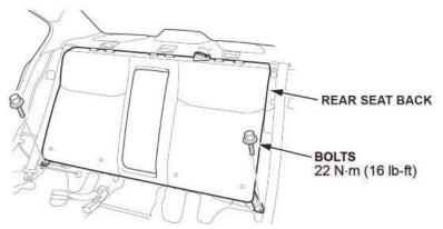
9. Lift the rear seat-back to release the wire loops with collars from the brackets.
