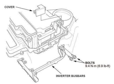
21. Remove the insulator, then remove the busbars.
