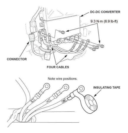
15. Remove the clip, ground cable, cables, and connectors from the PCU as shown.
