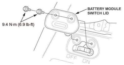
11. Turn the battery module switch to OFF, make sure you can see the bolt, then wait at least **5 minutes** to let the PDU capacitors discharge.
