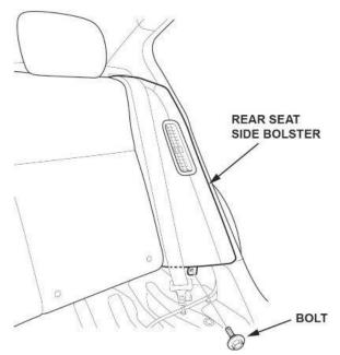
5. Remove the rear seat side bolster.
