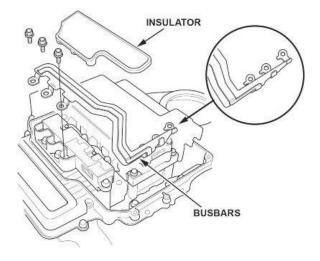
22. Remove the phase motor current sensor and the U, V, and W busbars.
