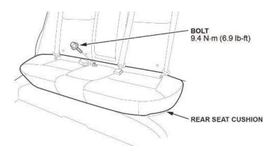
3. Push down on the rear seat cushion, pull out the seat hook handles to release the hooks, and remove the rear seat cushion.
