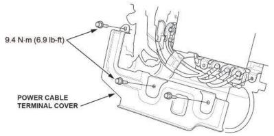
14. Disconnect the connector, then the four cables from the DC-DC converter, and wrap the end of the cables with insulating tape.
