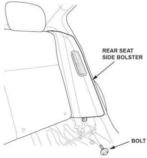
5. Remove the rear seat side bolster.
