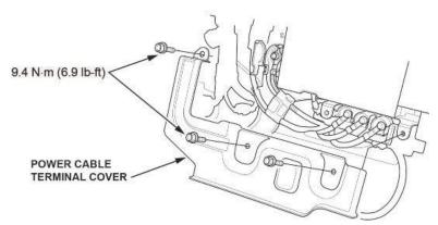
14. Disconnect the connector, then the four cables from the DC-DC converter, and wrap the end of the cables with insulating tape.
