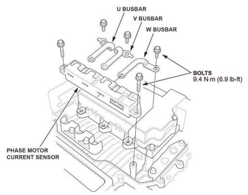
23. Remove the MPI module and install the new MPI module.
