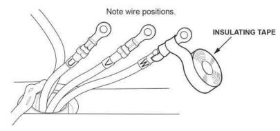
15. Remove the clip, ground cable, cables, and connectors from the PCU as shown.
