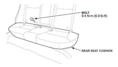
3. Push down on the rear seat cushion, pull out the seat hook handles to release the hooks, and remove the rear seat cushion.
