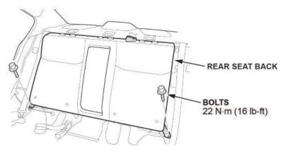
9. Lift the rear seat-back to release it from the seat legator hooks.
