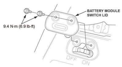
11. Turn the battery module switch to OFF, make sure you can see the bolt, then wait at least **5 minutes** to let the PDU capacitors discharge.
