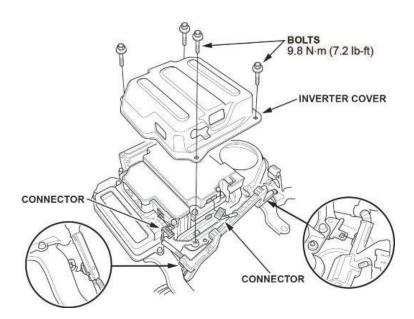
20. Remove the cover, then remove the IMA inverter busbars.
