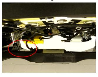
Make sure the seat mounting hardware is replaced and torqued as per the Repair Instruction.
