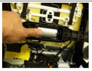
Remove the seat motor by pressing up from beneath.
