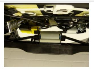
Remove the motor by sliding the drive cables out of both sides.
