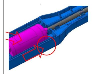
When seating the side with the electrical connector, slide the connector under a small tab as seen at left.
