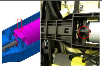
Reconnect seat motor electrical connector.
