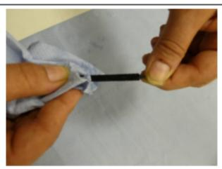
Lubricate the flexible drive shaft over its entire length using a lint-free cloth and P/N 83 23 9 407 810 Grease (NBU 12K)
